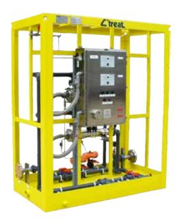
Designed for superior disinfection performance by providing a minimum 30,000  $\mu$ wsec/cm² UV dose at rated flow. The low-pressure, high-intensity (Lo-Hi) lamps are high power, monochromatic lamps offering up to three times the intensity of conventional Lo-Lo lamps at the optimum UV wavelength (254 nm) for disinfection. The performance is enhanced by a state-of-the-art electronic "smart" ballast and microprocessor control system.
